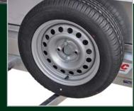
Optional WB103 spare wheel mounting bracket with WT760 195x70-14 spare wheel.
