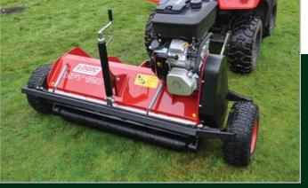
MFT120B18 seen here with standard wheels alongside. The height adjustment jack is spring assisted to make raising this very robust flail mower quite easy.
