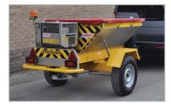
PDS hoppers are manufactured from stainless steel with a capacity of 585 litres (approximately 750kg). The mesh hopper screen, the sluice gate and the deflector vanes which allow salt to be cast to left or right are in common with the GDS range. Optional extras include a PDS208 tonneau cover, quick-attach PDS210 disc shroud and PDS106 flashing beacon.
