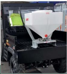
EBC-TS130PP 130 litre capacity, sized to fit a UTV, side by side, pick-up or compact tractor type vehicle where there is a significant area to cover whilst using an everyday vehicle as the means of travel.
