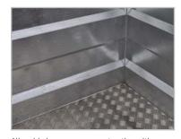
All-welded monocogue construction with aluminium 'tread plate' floor for safety, lighter weight benefits and easy cleaning for bio-security purposes.
