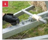
Lock the cradle onto the chassis.
