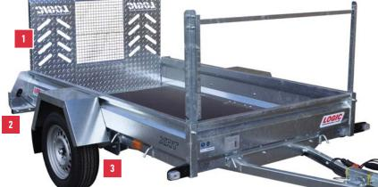
Optional lockable coupling with fitting kit, locking barrel and keys.
