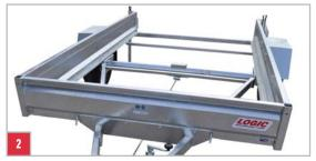
Monocoque construction with 'A' frame drawbar, Al-Ko suspension, one piece axle (1300kg) featuring rubber progressive action with excellent dampening. All protected with hot dipped galvanising for long life.
