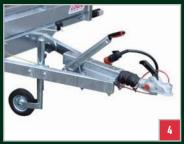
Overrun brakes with safety breakaway cable, handbrake and jockey wheel.
