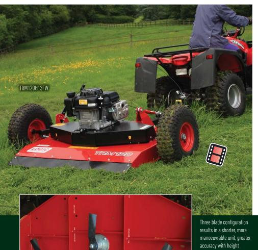
The Logic TRM120 is a compact rotary mower with three blades arranged to give a total working width of 1.2 metres which discharges cut material across the full width of the cutting deck. Cutting height can be adjusted in seconds and the height-adjustable drawbar means the TRM is just as happy behind a 4x4 as it is behind an ATV, utility vehicle or compact tractor. The drawbar can be offset for accurate edge work or cutting beneath overhanging vegetation.
