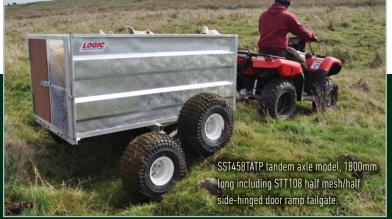
This tandem axle facility is useful on rough ground where every bump is evened out and especially when crossing a ditch or hole when carrying livestock. The easy carriage reduces stress on the animals and trailer, ensuring the life of the trailer is extended. In more extreme ground conditions, the wheel will flip over to climb out of a hole.
