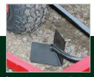
Options include a wheel track levelling kit (above) to enable one pass grading and a tine bar for rubber or bark surfaces, to level, agitate and reincorporate the surface.
