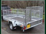
VT726 seen here with optional VT202 mesh extension sides and VT101 mesh headboard to 900mm high.
