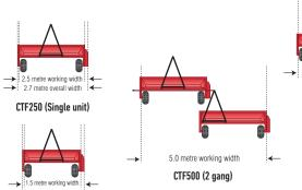
The CTF250 model is 2.5 metres wide with 22 x 11-8 low ground pressure wheels,
