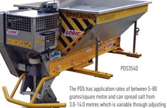
two available. The unit can spread salt to the left or right allowing it to spread underneath parked cars. Optional PDS211 disc shroud available.
