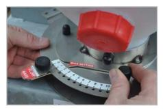
Bias setting: this adjustment is cleverly incorporated into the metering plate, compensating for the different characteristics of each type of product. In this way, even spreading can be consistently achieved.
