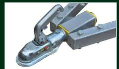
Swivel hitch - bolt-on, to permit fitting in one of 3 positions to match the towing vehicle.
