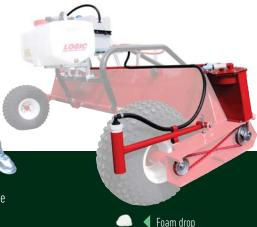
LBM100 bout marker is a very useful option especially where line of sight is obscured. This unit is ground driven from the Contact 2000 drive system and drops foam every few seconds. This makes an easy marker to follow to prevent overlapping or missing pieces.
