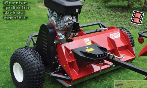
MFT120B18FW 'Scrub Buster' model fitted with optional flotation wheels.
