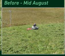
Glyphosate applied at a dilution rate of 20:1 with a work rate of up to 2.8Ha (7 acres) per hour using this 2.5 metre wide model. (Work rate dependent on forward speed, terrain and ground conditions).
