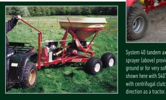
System 40 tandem axle fitted with spreader (left) or with sprayer (above) provide very stable units suitable for rough ground or for very soft conditions. Both applications are shown here with S40T13 models, featuring reverse drive with centrifugal clutch, to provide the same PTO rotation
