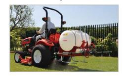
Perfect for small tractors with 'Cat 1' linkages like this compact tractor mower unit. The skid unit sets the sprayer at a good height for dismounting and storage.
