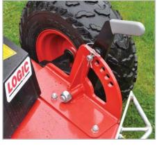
Cutting height adjustment can be carried out simply by moving the spring assisted height lever to one of 5 positions (from 20mm up to 160mm) and securing with the pin and clip.
