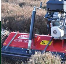
The adjustment of cutting height is controlled by a spring assisted screw jack giving cutting heights between 0-140mm on standard wheels and up to 216mm on flotation wheels.
