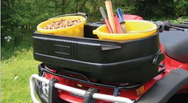
KOL91710 bucket hugger – a contoured cargo tray  $900 \times 450 \times 250$ mm designed to hold  $2 \times 25$  litre buckets. Constructed from double walled polypropylene with drain holes in the base, this is supplied with a mounting clamp and fittings or can be temporarily attached with bungee straps (not supplied).
