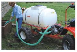
SLB620H has a Honda 2" diameter pump for discharge into elevated tanks or troughs. With a powered pump there is also an optional 5.0 metre suction hose kit which allows you to "self-fill" the bowser from any available fresh water source.
