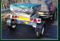
Model LMF610R with suspension axles, road wheels, lighting board and optional LMF101 tonneau cover.
