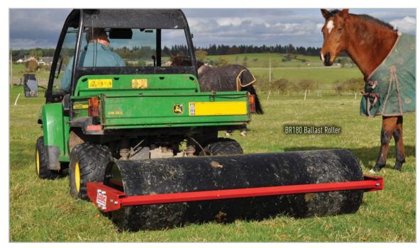
Used in conjunction with other soil preparation equipment, this unit is perfect for consolidating seed beds following reseeding or sowing game cover crops. These rollers feature a large diameter barrel which allows easy towing and a heavy wall section which prevents damage from stones. The weight can be altered by adjusting the water content to suit ground conditions and towing vehicle, to maintain good performance with safety on slopes, etc.
