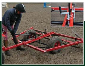
Easily operated over centre lever raises the Pro-Grade for transporting then lowers it into the work position. Inset picture shows the depth adjustment jack to set the blade to the best working level in various surfaces.
