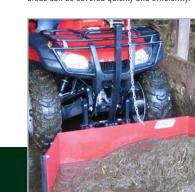
S210 yard scraper - suitable for cow sheds, cubicle houses, pig units, poultry houses, etc. With a working width of 1.3 metres, the heavy duty one piece blade is fitted with replaceable bottom and wing rubber wearing strips. Manual lift or electric ram options.
