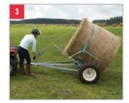
Winch the bale onto the chassis.
