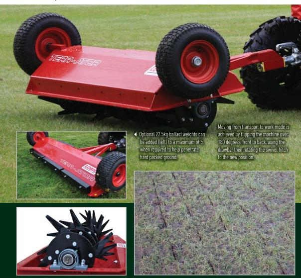
Detail of the 32 high-carbon steel blades, designed to penetrate ground with as little effort as possible.
