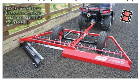
PG250 Pro-Grade provides quick and easy levelling of many types of surface. It features a perimeter plough to bring in material from the side of tracks or boards. It has low pressure tyres for all round capability and a raise and lower handle to lift the 2.5 metre blade clear of the ground for easy manoeuvring and transport as seen here below.
