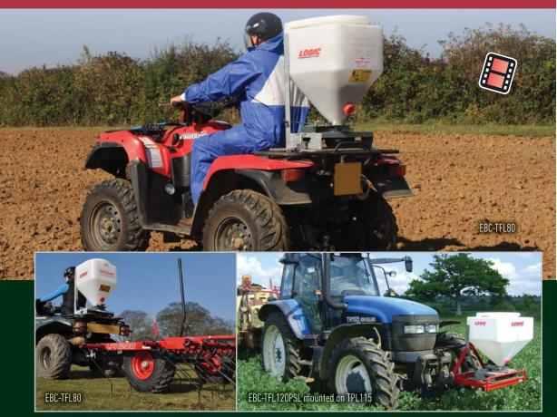
The range includes two hopper sizes of 85 litres (above) and 130 litres (above right). The 85 litre hopper is ideal for mounting on an ATV where high operational speed and low ground pressure can provide very high work rates. The 130 litre hopper gives extra capacity when used on larger vehicles such as UTVs, tractors and self-propelled sprayers.
