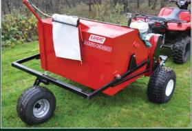
This model features a 600 litre capacity hopper with tipping rope and single pivot point. The contents would typically be tipped onto a tarpaulin or sheet for further processing before drying and cleaning (as shown right)
