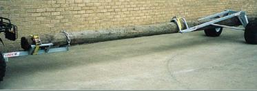
PB800 pole bogie used with an ATV, UTV, Land Rover or similar vehicle, can transport difficult objects like long poles with ease. Its design features adjustable gripping chain and removable drawbar to handle practically any length of pole or pipe, etc. Easy to attach with no other equipment required.
