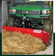
UTS210 yard scraper - suitable for cow sheds, cubicle houses, pig units, poultry houses, etc. With a working width of 1.7 metres, the heavy duty, one piece blade is fitted with replaceable bottom and wing rubber wearing strips. Raise and lower is operated from inside the cab with the remote controlled electrical actuator.
