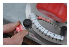
Flow rate adjustment: the unique metering plate mechanism is key to this reliable and accurate system. Twin feed apertures allow for large and small products to be successfully handled – even when a very low application rate is required.
