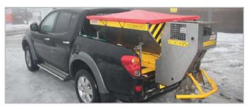
The de-mount version can be secured into a pick-up, flat bed truck or onto a trailer. Importantly, the de-mount version has a gross weight of 1000kg which allows it to be used in pick-ups and other vehicles. This makes use of an existing fleet vehicle as a professional salt spreading asset.
