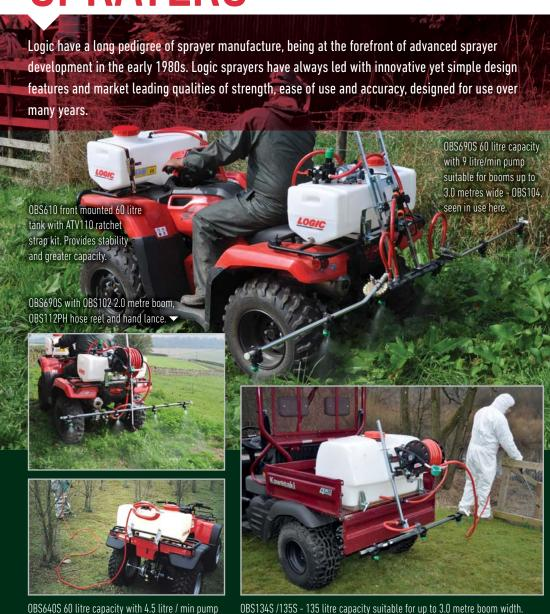
OBS134S /135S - 135 litre capacity suitable for up to 3.0 metre boom width. Ideal for larger ATVs, UTVs, 4x4s, etc. Seen here with OBS112PH 15.0 metre hose reel with hand lance and OBS101 1.5 metre boom
