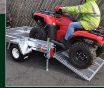
XRT610E with 20.5x8-10 wheels and tyres with optional XT106 mesh ramp tailgate and RT710-02 rear prop stands. Ideal for transporting an ATV or garden tractor.
