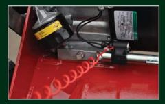
A safety kill switch and lanyard provide an instant engine stop facility for any hazardous situation eq. wire wrapping around the blades.
