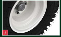
Bead-lock wheel rims provide additional security for tyre to rim adhesion, particularly as these tyres operate at low pressure.
