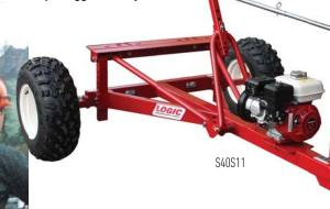
System 40 chassis provides a low ground pressure option for tractor sized equipment. Existing spreaders and sprayers are simply bolted onto the unique cross member of this universal chassis. It features an adjustable axle track width, adjustable equipment platform height, a manual ON/OFF handle, flotation wheels and a 5.5hp Honda engine with PTO type interface.
