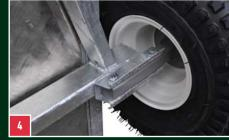
Bolt-in stub axles allow easy replacement when the time comes. This method ensures the galvanising protection is <u>not disturbed. These trailers are desig</u>ned to last a long time!
