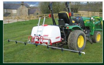
DMS390S with optional DMS303 boom mounting bracket fitted to the side of the frame to allow fitting into smaller UTV cargo beds or other carrying systems, shown here with OBS102 2.0 metre boom.
