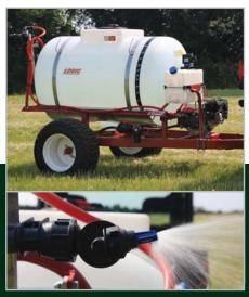
TS625 sprayer is a boomless model using one or two Hypro XT020 broadcast nozzles to produce spray widths of up to 11.0 metres with application rates up to 285 litres/ha. Ideal for spraying areas where a conventional boom is not practical.
