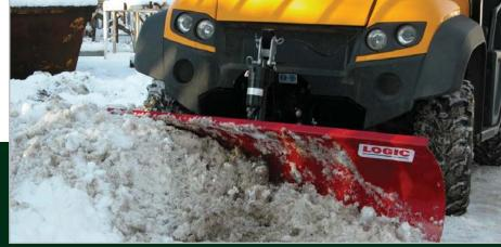
UTS201 snow plough - the extra width and power of a UTV means that the blade can be wider than ATV snow ploughs this unit is 1.8 metres. The supplied in-cab controlled, 12v electric ram provides the raise and lower facility. The snow plough can be manually angled to either side and is suitable for clearing snow up to 300mm in depth. Safety features include a rubber wearing strip and spring loaded 'break-back' system which operates if the blade should hit an obstacle hidden beneath the snow.
