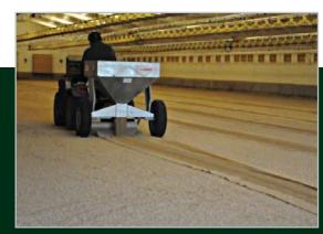
This basic LCF160 lays out approximately 1500kg of feed on 6 rows of paper in this broiler house in 5 minutes (plus filling time) a fraction of the time of previous methods.
