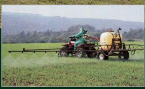
TS500/600 based on the well proven Hardi sprayer, with self-levelling booms of 10.0 -12.0 metre widths. These models are mounted in a sturdy chassis with an engine driven pump providing a stable low ground pressure unit.
