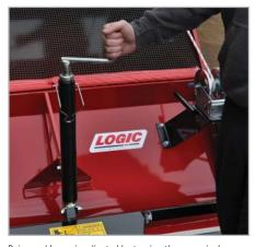
Raise and lower is adjusted by turning the screw jack handle which offers very fine adjustments. This gives a very accurate height control of the brush which is good for all surfaces, particularly short, fine piles.
