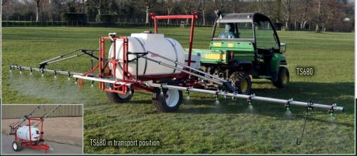
TS660/680 sprayers feature the same strong, rotationally moulded, translucent, polyethylene 600 litre tank, mounted on a sturdy 'A' frame chassis with low ground pressure 23 x 10.5-12 wheels and tyres. Output is supplied from a Honda engine, 25 litre/min diaphragm pump controlled by remote electric ON/OFF and manual pressure regulation. A 15 litre clean water tank is mounted to comply with Health & Safety regulations.
