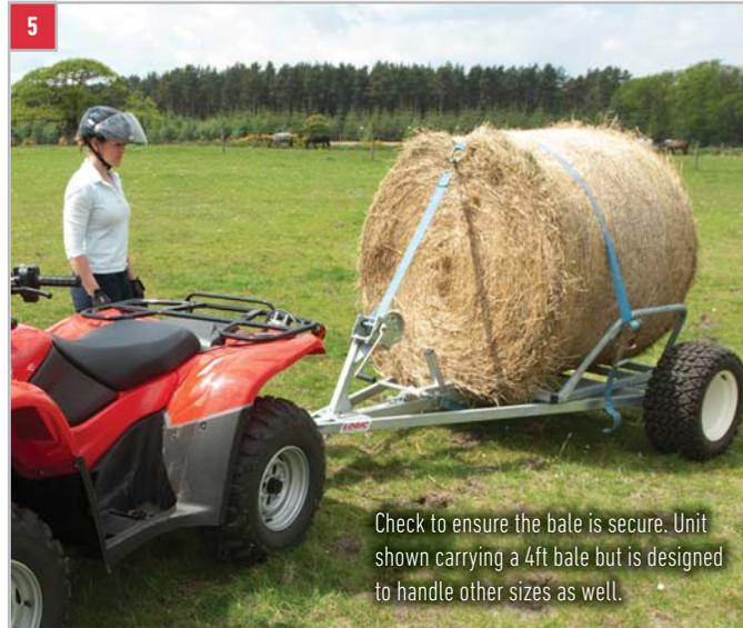
5 Check to ensure the bale is secure. Unit shown carrying a 4ft bale but is designed to handle other sizes as well.
