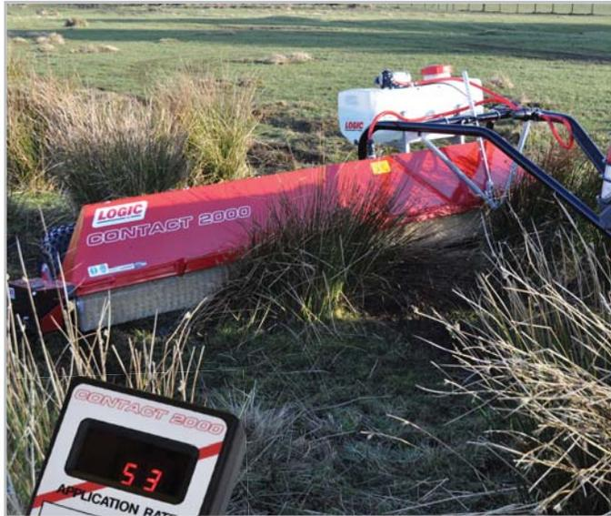
Hands-free operation without any complicated electrics or sensors, this easy to use control box allows the operator to select the required rate for the level of weed infestation being treated, ensuring the lowest possible usage of chemical to achieve the desired results. An override button allows the operator to instantly increase the amount of chemical delivered should there be a dense patch of weeds in an otherwise sparse infestation.
