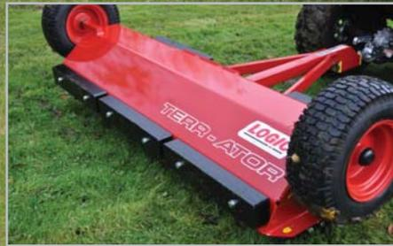
◀ Optional 22.5kg ballast weights can be added (left) to a maximum of 5, when required to help penetrate hard packed ground.
