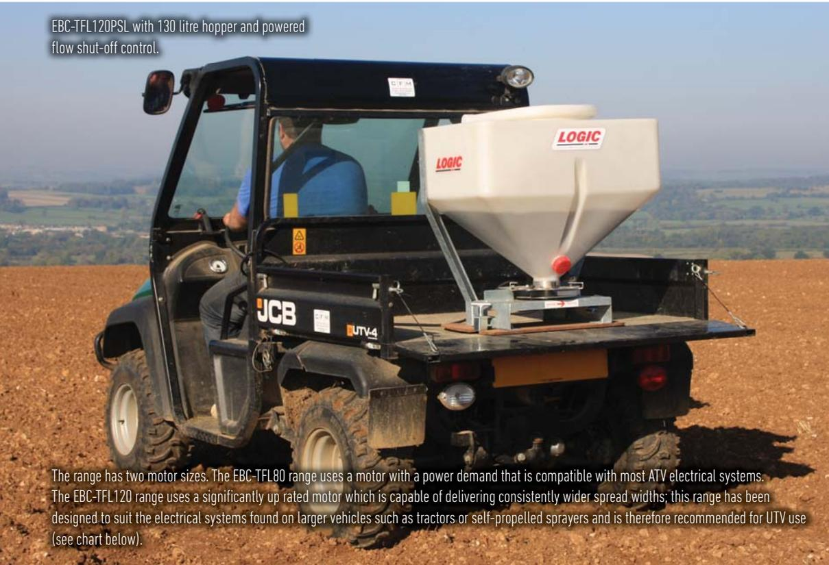
The range has two motor sizes. The EBC-TFL80 range uses a motor with a power demand that is compatible with most ATV electrical systems. The EBC-TFL120 range uses a significantly up rated motor which is capable of delivering consistently wider spread widths; this range has been designed to suit the electrical systems found on larger vehicles such as tractors or self-propelled sprayers and is therefore recommended for UTV use (see chart below).
