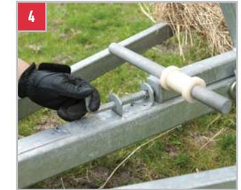
4 Lock the cradle onto the chassis.
