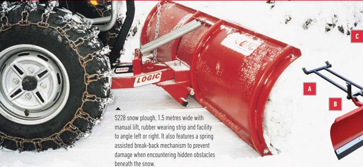
▲ S228 snow plough, 1.5 metres wide with manual lift, rubber wearing strip and facility to angle left or right. It also features a spring assisted break-back mechanism to prevent damage when encountering hidden obstacles beneath the snow.
