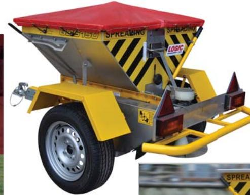
GDS150R (left) with optional GDS158 tonneau cover is the smallest in the GDS range and is designed to be towed by smaller vehicles such as an ATV or UTV. It features a stainless steel hopper and peripheral components to give a spread width of 1.5-12.0 metres at 4-15mph. Options include GDS106 flashing beacon, GDS158 tonneau cover and quick-attach PDS210 disc shroud to restrict spread width to 1.5 metres without reducing forward speed (also fits GDS200 / 250 models).
