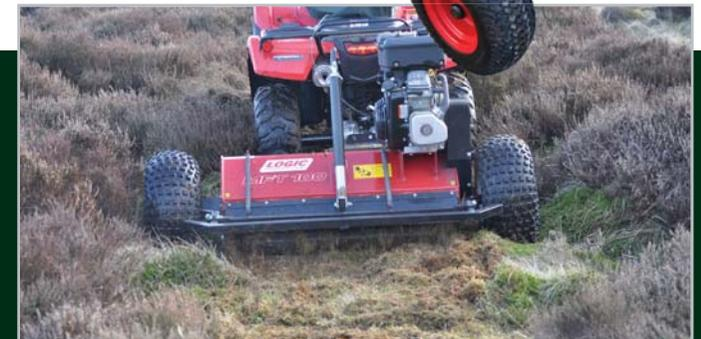
Flotation wheels are a useful option for soft or rough ground and are always recommended when cutting heather, seen here (above) cutting fire breaks on an upland grouse moor.
