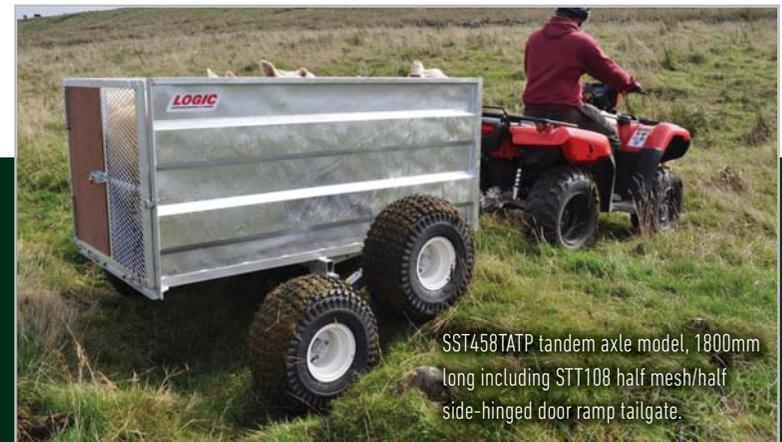
SST458TATP tandem axle model, 1800mm long including STT108 half mesh/half side-hinged door ramp tailgate.
