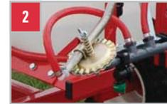
Adjustable break-back clutch for boom safety and protection.
