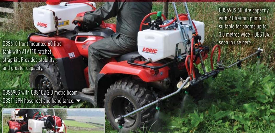
OBS610 front mounted 60 litre tank with ATV110 ratchet strap kit. Provides stability and greater capacity.
