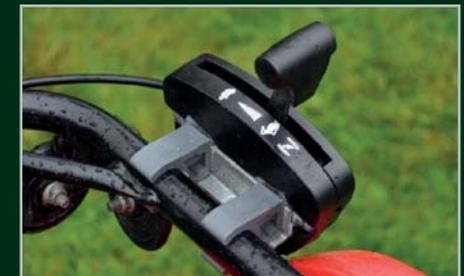
The remote throttle gives control from the operator's driving position.
