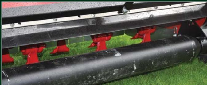
The full width anti-scalping roller (above) protects the sward from scalping and allows cutting over kerbs, etc.
