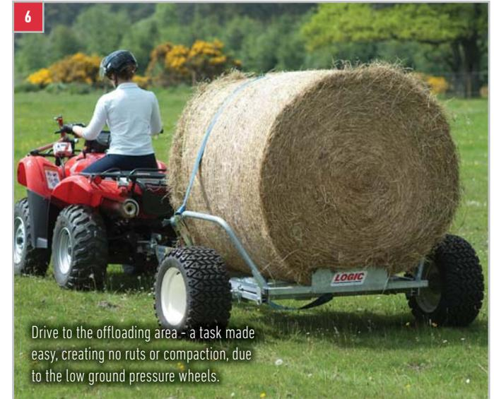
6 Drive to the offloading area - a task made easy, creating no ruts or compaction, due to the low ground pressure wheels.
