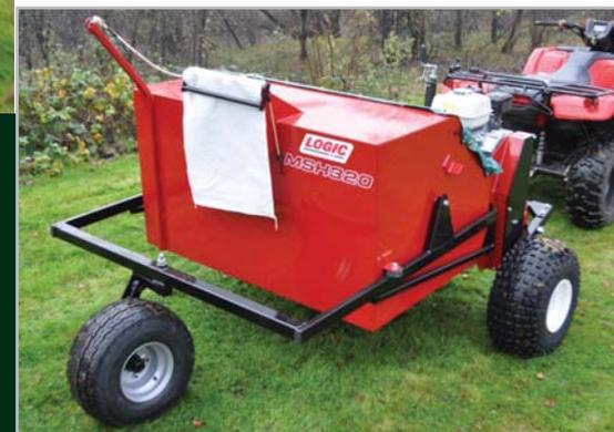
This model features a 600 litre capacity hopper with tipping rope and single pivot point. The contents would typically be tipped onto a tarpaulin or sheet for further processing before drying and cleaning (as shown right).
