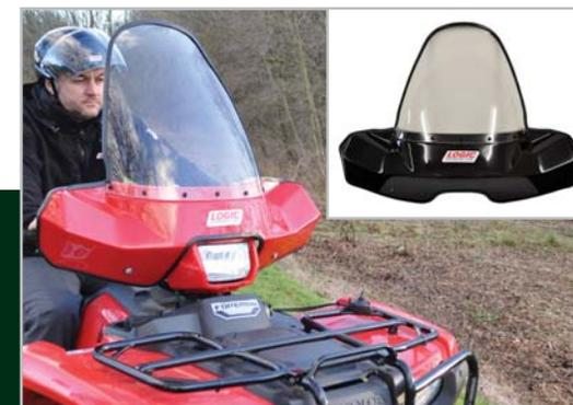
Logic ATV074/77/XXX windscreens have been specially designed for ATVs, incorporating a stylish fibreglass handlebar fairing which creates an effective brush guard and protection from wind chill. The screens are made from durable 4mm cast acrylic with edge trim for added safety. Colour choice is red or black.
