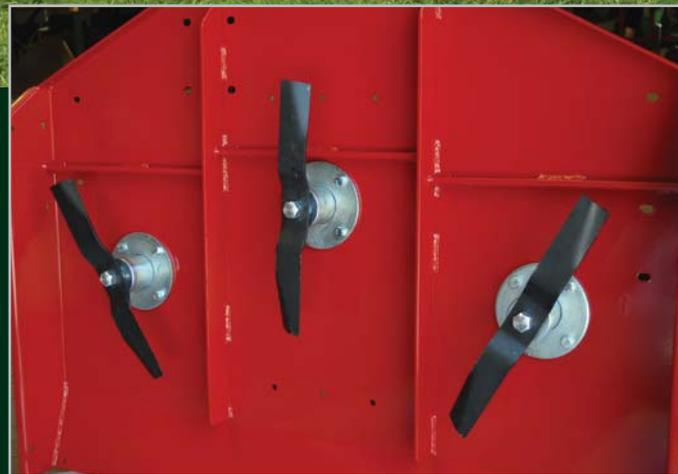
Three blade configuration results in a shorter, more manoeuvrable unit, greater accuracy with height adjustment and less tendency to scalp over rises. The engine power is used more effectively so fuel usage should be reduced and any blade damage minimised.
