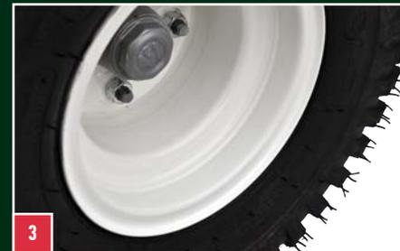
Bead-lock wheel rims provide additional security for tyre to rim adhesion, particularly as these tyres operate at low pressure.
