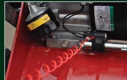
A safety kill switch and lanyard provide an instant engine stop facility for any hazardous situation eg. wire wrapping around the blades.
