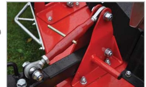
Drawbar top link adjustment is carried out to level the cutting deck to suit whichever vehicle is being used to tow the mower. The offset facility on the drawbar is useful when cutting under overhanging vegetation.
