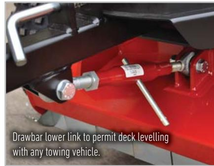
Drawbar lower link to permit deck levelling with any towing vehicle.
