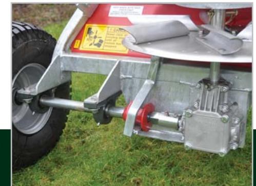
There are few moving parts on this spreader range and maintenance is minimal. The quality galvanised finish ensures the chassis and mounting frame will last for many years.
