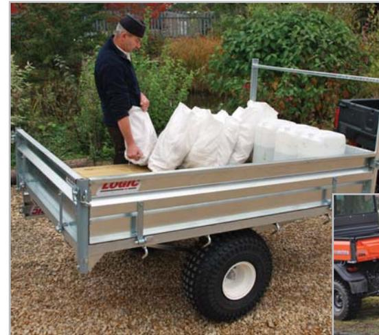
DST400 flat bed trailer (left) 1970 x 1400mm with standard ladder rack, seen here with optional DST103 300mm drop side kit. This trailer has a huge carrying area suitable for bags or bales with an easy loading height. Optional DST106 mesh sides and rear door extension kit and DST105 solid panel headboard to 800mm are available (below).
