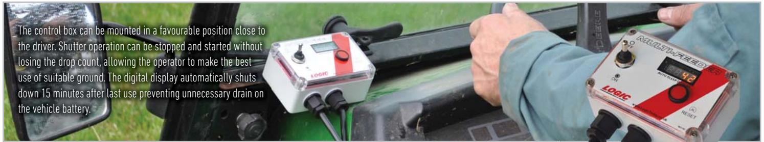
The control box can be mounted in a favourable position close to the driver. Shutter operation can be stopped and started without losing the drop count, allowing the operator to make the best use of suitable ground. The digital display automatically shuts down 15 minutes after last use preventing unnecessary drain on the vehicle battery.
