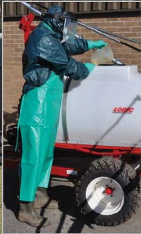
TS400S trailed sprayer with 270 litre capacity tank and a choice of 4.5 or 9 litres / min pump to be used with optional booms from 1.5 metres to 3.0 metres, single broadcast nozzle, hand lance and 15.0 metre hose reel.
