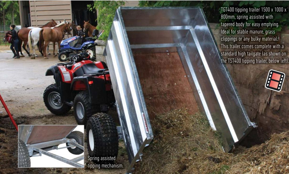
TGT400 tipping trailer 1500 x 1000 x 800mm, spring assisted with tapered body for easy emptying. Ideal for stable manure, grass clippings or any bulky material. This trailer comes complete with a standard high tailgate (as shown on the TST400 tipping trailer, below left).
