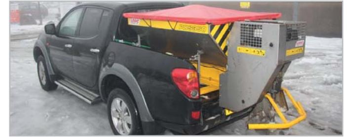
PDS hoppers are manufactured from stainless steel with a capacity of 585 litres (approximately 750kg). The mesh hopper screen, the sluice gate and the deflector vanes which allow salt to be cast to left or right are in common with the GDS range. Optional extras include a PDS208 tonneau cover, quick-attach PDS210 disc shroud and PDS106 flashing beacon.
