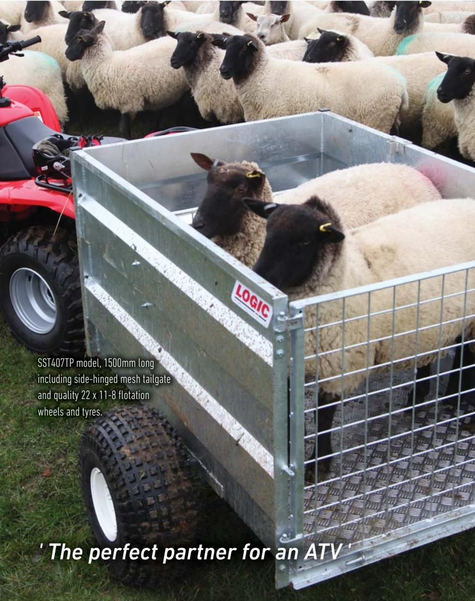
SST407TP model, 1500mm long including side-hinged mesh tailgate and quality 22 x 11-8 flotation wheels and tyres.
