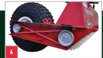
The contra-rotating brush is ground driven from the wheel using a segmented 'V' belt housed under a robust, protective cover. Low ground pressure tyres on bead-lock rims allow for use in soft, wet ground and provide suspension for the unit when working in rough conditions.
