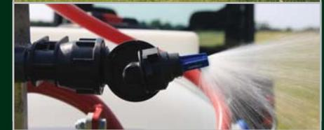
TS625 sprayer is a boomless model using one or two Hypro XT020 broadcast nozzles to produce spray widths of up to 11.0 metres with application rates up to 285 litres/ha. Ideal for spraying areas where a conventional boom is not practical.
