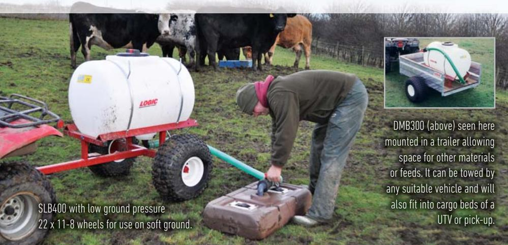
SLB400 with low ground pressure 22 x 11-8 wheels for use on soft ground.
