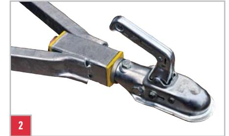
50mm swivel ball hitch provides a robust, safe coupling with articulation for travelling over rough ground. This is a recommendation by the Health & Safety Executive. Other hitch types such as clevis, 40mm ring, etc. are available.
