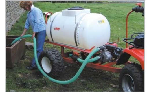
SLB620H has a Honda 2" diameter pump for discharge into elevated tanks or troughs. With a powered pump there is also an optional 5.0 metre suction hose kit which allows you to "self-fill" the bowzer from any available fresh water source.
