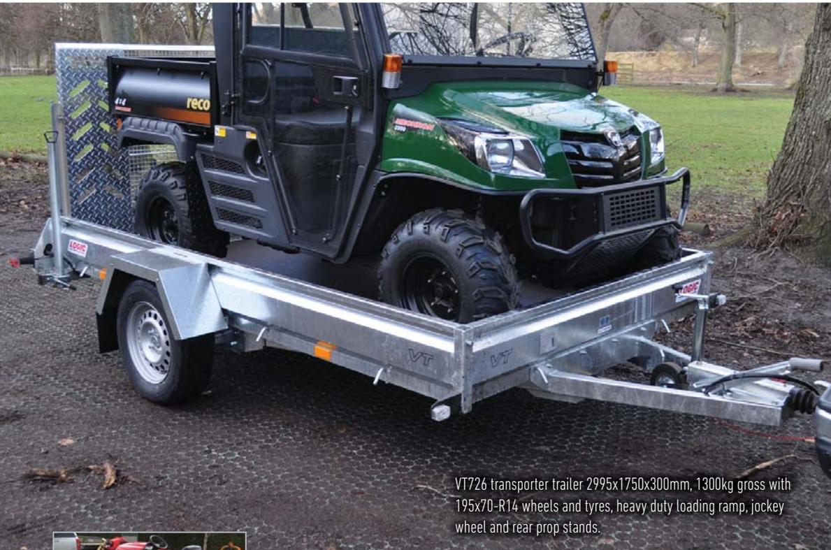
VT726 transporter trailer 2995x1750x300mm, 1300kg gross with 195x70-R14 wheels and tyres, heavy duty loading ramp, jockey wheel and rear prop stands.
