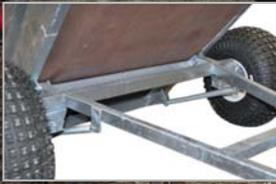
Spring assisted tipping mechanism.
