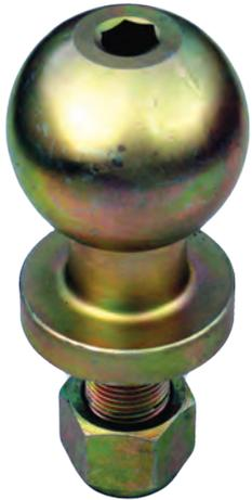
TB100 tow ball (left). Standard features include: 50mm diameter, short 3/4" thread with Nyloc nut, 10mm allen key slot to assist fitting. Designed specifically for ATVs and UTVs.
