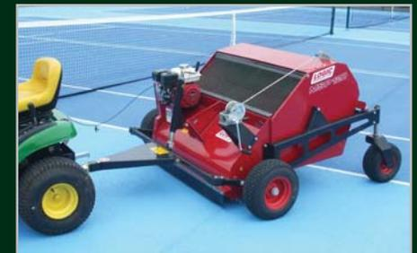
The MSP120W (above) seen here sweeping all weather tennis courts, keeps the surface clear of dust, grit and other debris. In this case it is towed by a ride on lawnmower.
