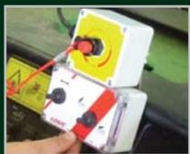
A wired control box operates the 12v actuator ram which raises and lowers the front mounted equipment and includes the added safety feature of an engine kill switch. This can be positioned close to the operator using the ample amount of cable provided.
