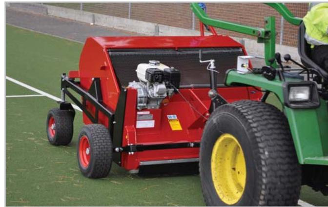
On fine, dense artificial surfaces with very little pile, grit, leaves and particularly pine needles can become a problem. With the MSP these can be cleared up very quickly and the sweeping action helps break up any crusts or mould.
