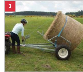
3 Winch the bale onto the chassis.
