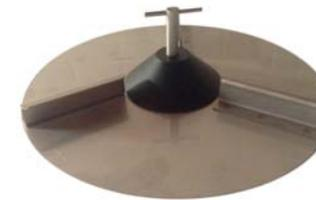
Low impact delivery system - this central cone, unique to Logic machines, reduces the impact of the product hitting the high-speed spinning disc (left). When slug pelleting or spreading fertiliser this minimises 'dusting' (when the product breaks up on impact with the disc). It is also a major benefit when broadcasting seeds, as they are protected from damage compared with some other systems. This leads to higher germination rates.
