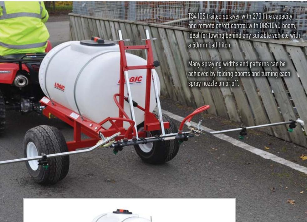
TS410S trailed sprayer with 270 litre capacity and remote on/off control with OBS104D boom, ideal for towing behind any suitable vehicle with a 50mm ball hitch.
