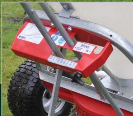
Adjustable flow control can be operated from the driving position on ATVs. Disc drive engagement is extremely simple and can be disengaged when not spreading.
