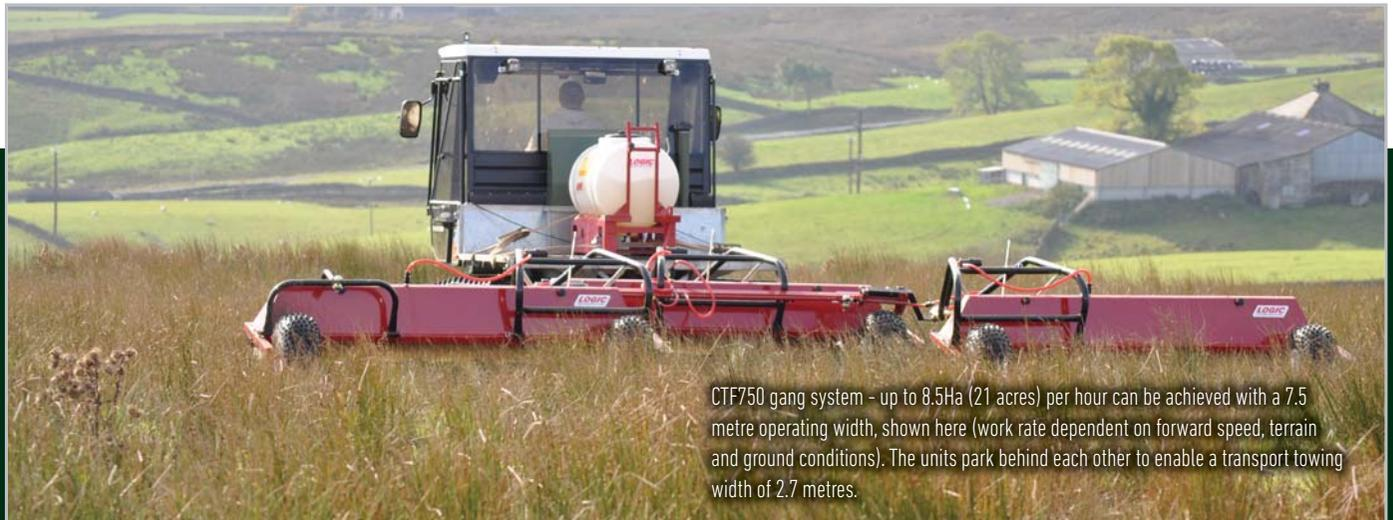
CTF750 gang system - up to 8.5Ha (21 acres) per hour can be achieved with a 7.5 metre operating width, shown here (work rate dependent on forward speed, terrain and ground conditions). The units park behind each other to enable a transport towing width of 2.7 metres.
