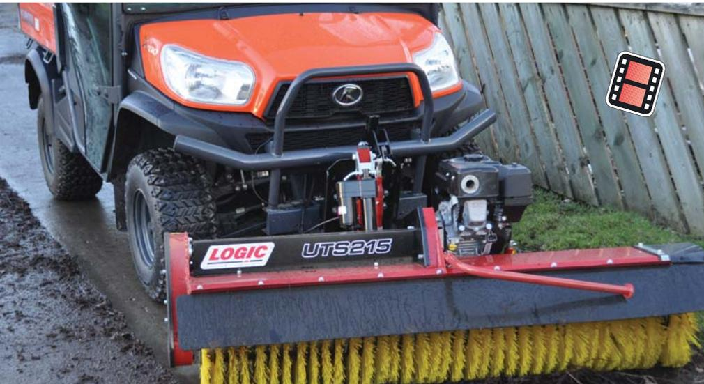
UTS215BR power brush - 1.68 metres wide with remote electric controls to lift and angle left, right or straight. Shown here with a Briggs & Stratton 6.5hp petrol engine. The UTS215HR model features a Honda 5.5hp petrol engine.
