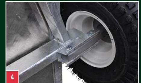
Bolt-in stub axles allow easy replacement when the time comes. This method ensures the galvanising protection is not disturbed. These trailers are designed to last a long time!
