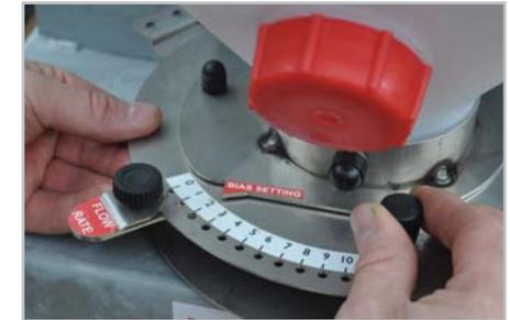
Bias setting: this adjustment is cleverly incorporated into the metering plate, compensating for the different characteristics of each type of product. In this way, even spreading can be consistently achieved.
