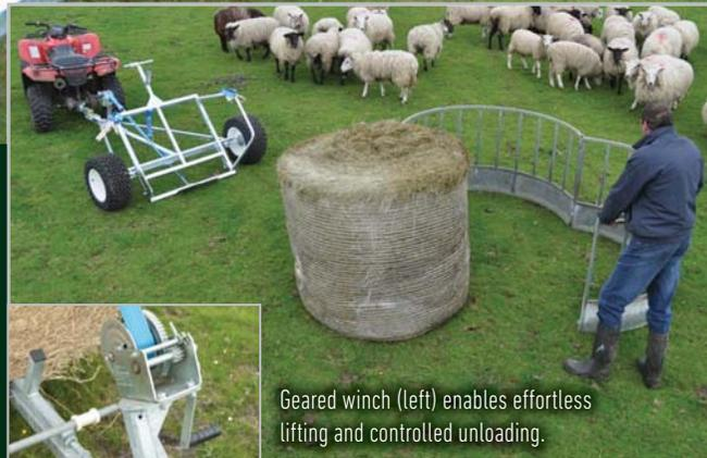
Geared winch (left) enables effortless lifting and controlled unloading.
