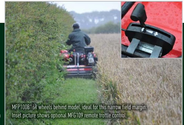
MFP100B16R wheels behind model, ideal for this narrow field margin. Inset picture shows optional MFG109 remote throttle control.
