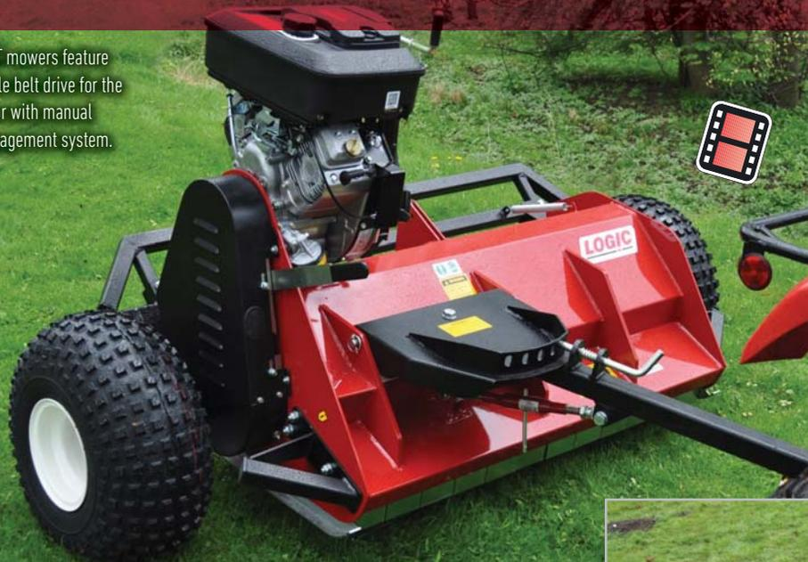
MFT120B18FW 'Scrub Buster' model fitted with optional flotation wheels.
