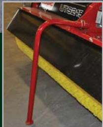
UTS215 parking leg - allows the power brush to be stored without the bristles taking any weight therefore preventing distortion of the brush. This prolongs the life of the brush bristles and permits more stable parking.
